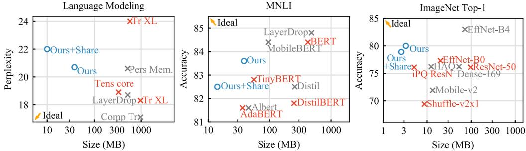
Figure 2: **Performance as a function of model size.** We compare models quantized with PQ and trained with the related Quant-Noise to the state of the art. (a) Test perplexity on Wikitext-103 (b) Dev Accuracy on MNLI (c) ImageNet Top-1 accuracy. Model size is shown in megabytes on a log scale. Red and gray coloring indicates existing work, with different colors for visual distinction.
