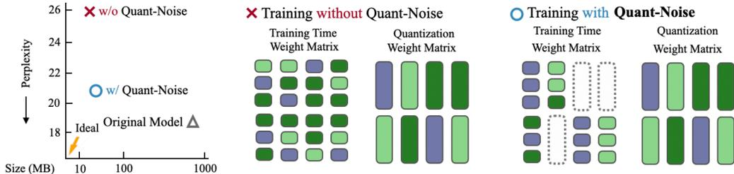
Figure 1: **Quant-Noise** trains models to be resilient to inference-time quantization by mimicking the effect of the quantization method during training time. This allows for extreme compression rates without much loss in accuracy on a variety of tasks and benchmarks.
